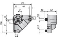
Screw-fix/dowel-fix 1 Ø12 pivot pin mounting base.
