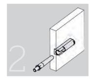
The base provides a flange for positioning on the edge of the furniture. Secure the Ø3x12 screw and then introduce the damper on the front.
