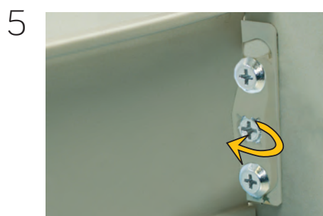
This drawer front fixing bracket will allow a vertical adjustment of +/-2mm.
